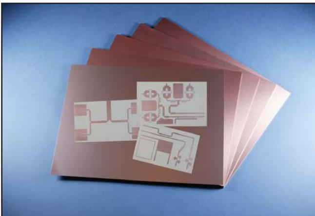
Standard tolerance dielectric thicknesses of 0.010", 0.025", 0.050", 0.075", and 0.100" (0.254, 0.635, 1.270, 1.905, 2.54 mm) are available. When ordering RT/duroid 6006 and RT/duroid 6010LM laminates, it is important to specify dielectric thickness, electrodeposited or rolled, and weight of copper foil required.
